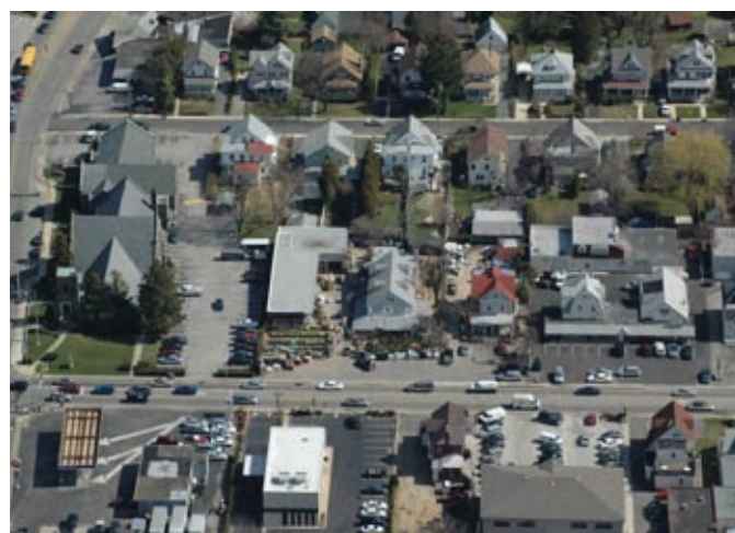
Wide Curb Cut Along Eagle Road Increases Vehicular and Pedestrian Conflicts
